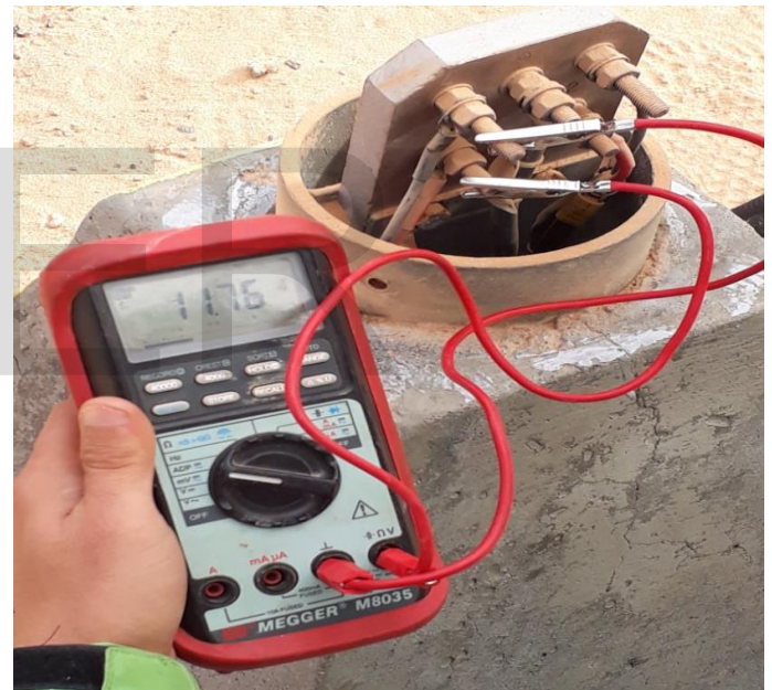
Figure 2.1. High input impedance digital voltmeter
