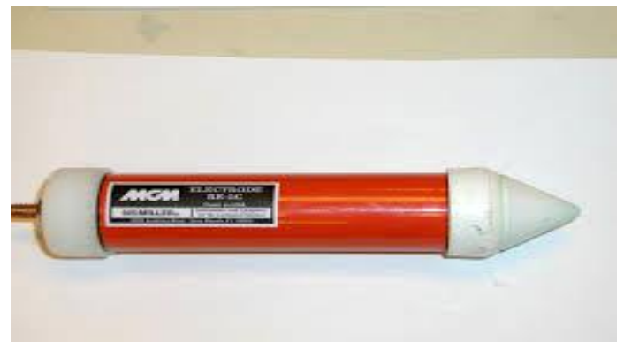
Figure 2.2. Cu-CuSO 4 half-cell electrode
